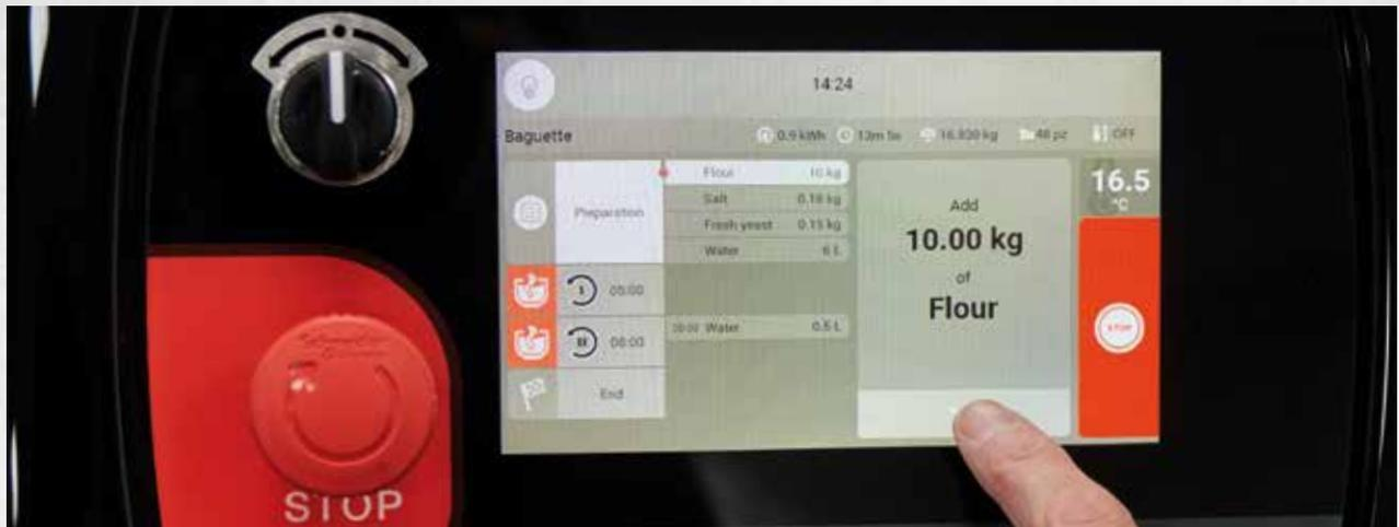
The Recipe mode provides **step-by-step instructions** for the mixing process. The user can program resting times and set reminders to add ingredients.
