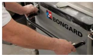
A grip handle that protects the control knobs and allows safe moving of the divider
